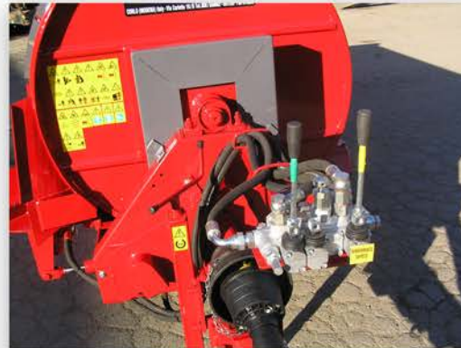
Impianto idraulico indipendente con pompa e serbatoio. Independent oil circuit with pump and oil tank.
